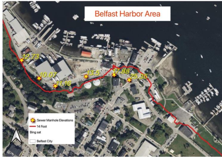
Figure 1 Aerial Photo Map of Front Street showing the 14 foot elevation contour line if sea level rises as predicted by 2050.
